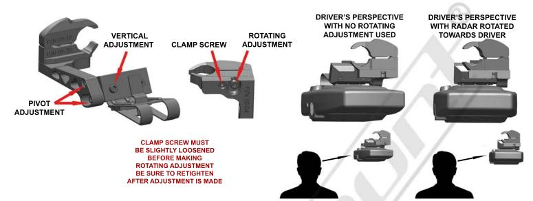
**STEP 3** - Install your radar detector onto the mount. Use the adjustments shown above to adjust the RD to your desired position. We recommend adjusting the RD as close to the bottom of your mirror as you can. **NOTE** When the rotating adjustment is used to rotate the RD towards the driver, the footprint of the RD is reduced as shown above. Be sure to tighten all of the adjustment screws after the adjustments are made.
