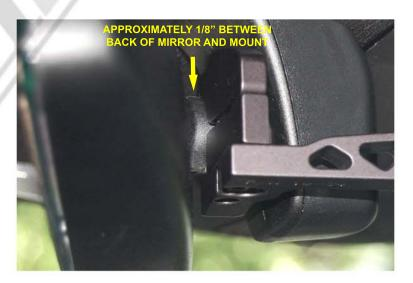
**STEP 1** - Loosen the clamp screw so the top section separates from the mid section. This will provide the necessary clearance to slide the mount over the mirror stem as shown above.
